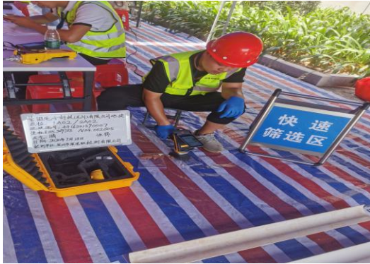
1A02-土壤挥发性有机物样品取样
