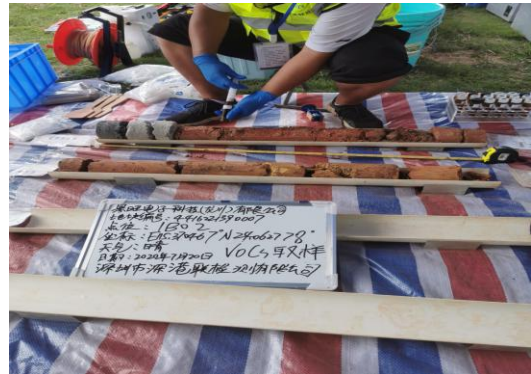
1B02-土壤挥发性有机物样品取样
