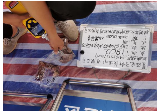
1B02-土壤挥发性有机物样品取样
